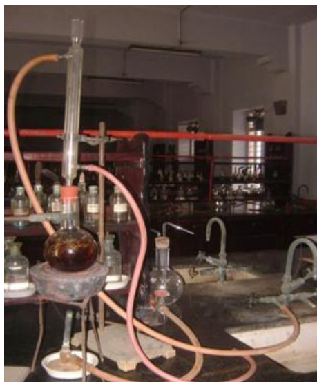
Figure 2 Photograph of experimental set up for obtaining plant extract using reflux condenser
