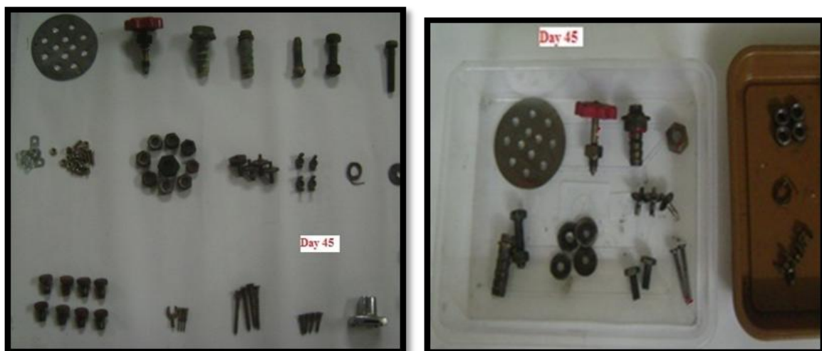
Figure 5. Photograph of (a) untreated and (b) treated metal parts on day 45 of Atmospheric exposure
